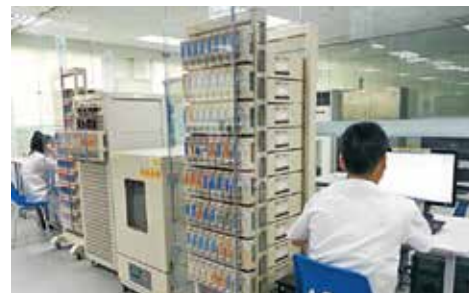
Cyclic charge and discharge testing machine
